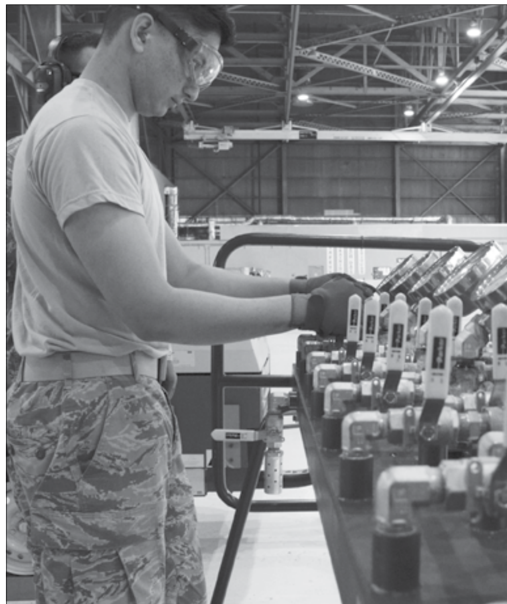
U.S. Air Force photo/Senior Airman Amber Carter Senior Airman Raunak Manandhar, 60th Maintenance Squadron aero repair technician, monitors the pounds per square inch while inflating lifting bags during an annual quality assurance inspection of the Crash, Damaged or Disabled Aircraft Recovery program Feb. 9 at Travis Air Force Base, Calif.
